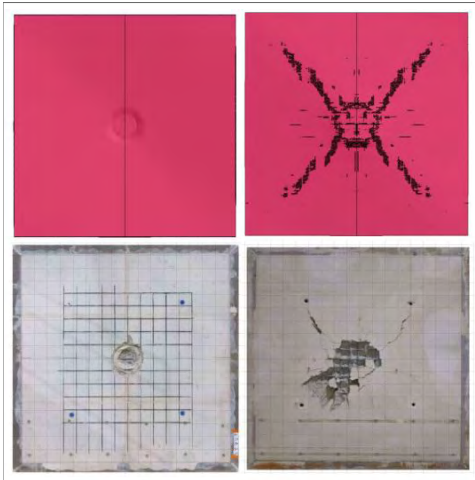
Figure 7: Crack and damage pattern for GSX1R-L test and simulation [3].
