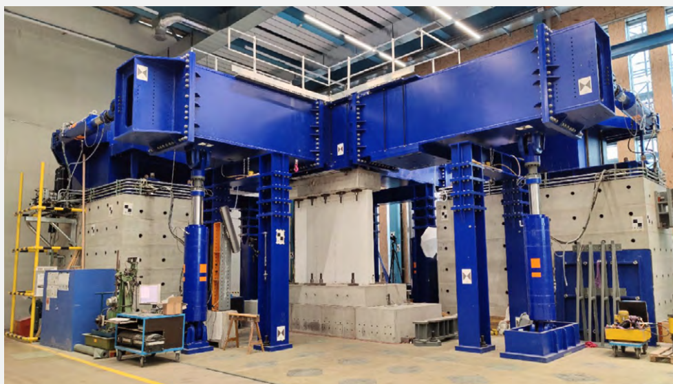
Figure 3: ETH MAST Facility. Testing of a squat rectangular RC wall conducted by Pizarro [1].
