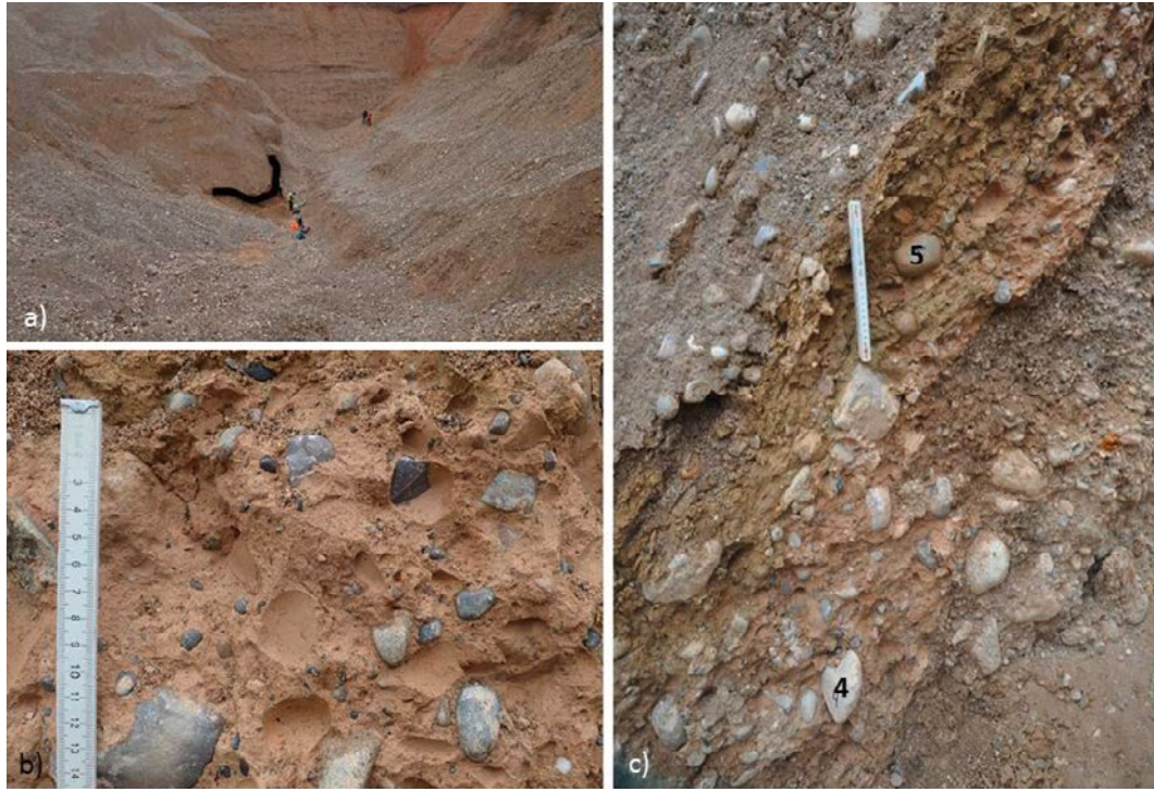
Figure 2: a) Picture of the gravel pit in Möhlin. Black line shows the inclined layer of the Bünnten till. b) Photo of the Bünnten Till exposed in the gravel pit. c) Samples (labelled with 4 and 5) taken from the Bünnten Till.
