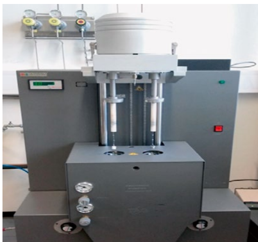
Figure 2: Setaram TAG facility for SETs
