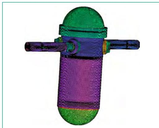
Figure 6: Structured mesh of the RPV for CFD.
