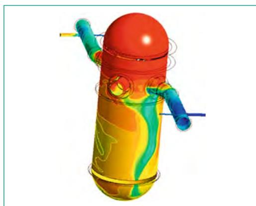
Figure 7b: Temperature distribution at the inner RPV wall for the MBLOCA at  $t = 29$  s.
