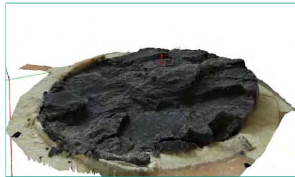
Figure 6: 3-D model of a typical failure surface from the CNS tests.
