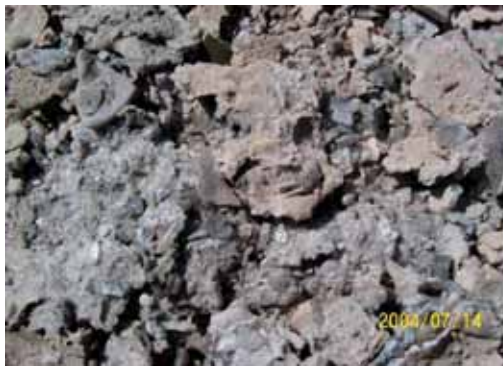
Figure 2.9: Structure of debris upper layer from COMECO top-flooding tests.
