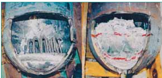
Figure 2.5: The in-vessel configurations of the FOREVER-EC4 test (left; failed vessel) and EC5 test (right; non-failed vessel).
