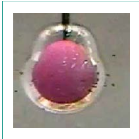
Fig. 4.8: The image of the 10mm heated sphere during film boiling in pure water at the liquid subcooling of 70 ~ 81 K
