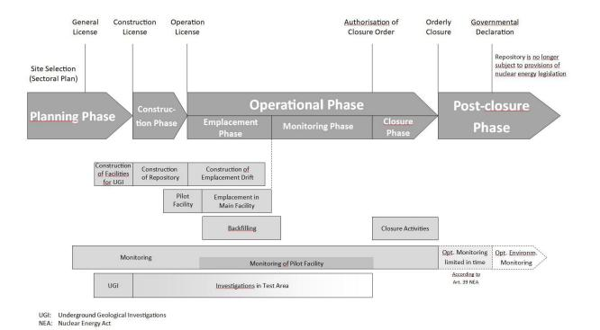
The operational phase of a deep geological repository comprises waste emplacement, the monitoring phase and closure.
