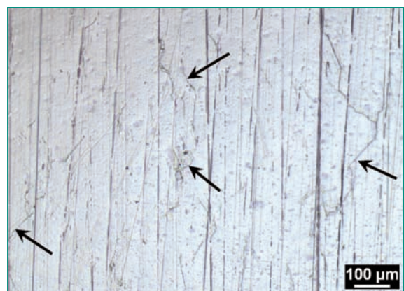
Fig. 27: Same fatigued specimen as in Fig. 26: Replica from machined surface. Machining grooves and short cracks. Poor contrast between grooves and cracks ( \leftarrow ).
