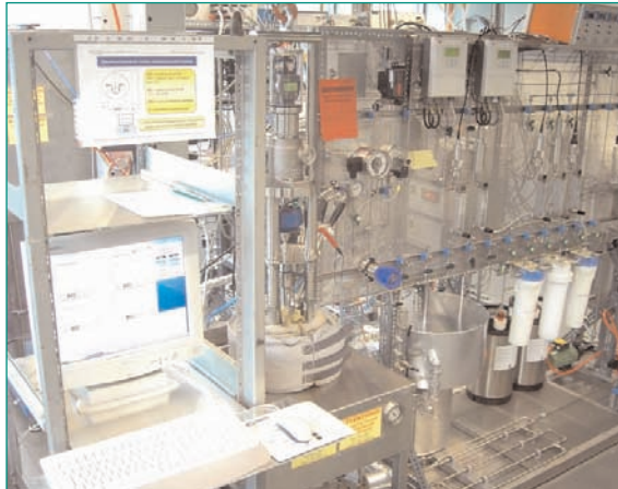
Figure 10: a) High-temperature water loop and autoclave with integrated electro-mechanical tensile loading machine with EN measurement system for SCC initiation studies under BWR/NWC conditions. b) schematic of used cell configuration for simultaneous electrochemical potential (EPN) and current noise (ECN) measurements (with a zero resistance ammeter (ZRA)) in autoclave.
