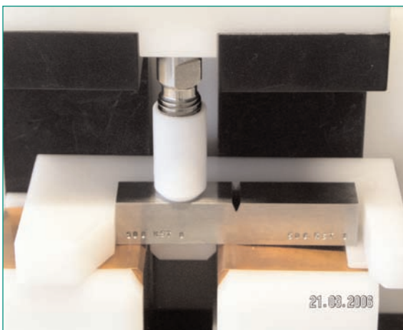
Fig. 42: Clean, unbroken Charpy specimen mounted on the TEP device.
