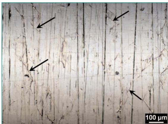
Fig. 26: TP 304L (A), low cycle fatigued: \Delta\epsilon_f/2 = 0.3\% , T = 200^\circ\text{C} , D = 1.0 , N = 29'740 [1]. Machined surface. Machining grooves and short cracks. Poor contrast between grooves and cracks ( \leftarrow ).
