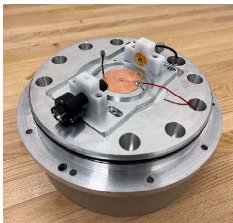
Figure 3: Detector lid of new prototype. The alpha beam gets collimated (black parts) and detected by the surface barrier detector (golden part). The ions travel towards the dielectric plate hole (hole in center of copper area) and the electron avalanche is detected on the signal read out pad (copper area connected to red cable).
