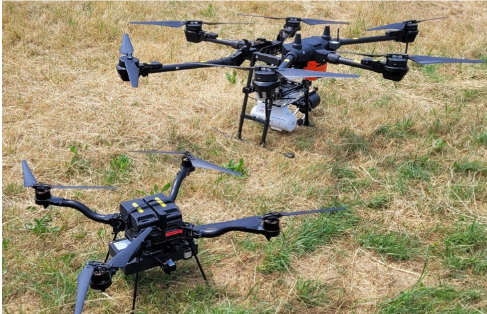
Figure 3: Drones with attached measuring systems used during the ARM23c source search exercise (front: Arktis Radiation Detection Ltd, back: Spiez Laboratory/ armasuisse).
