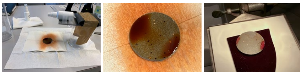
Figure 1: Five-cm diameter rubber flooring circles contaminated by simple spraying from 11.5 cm distance.
