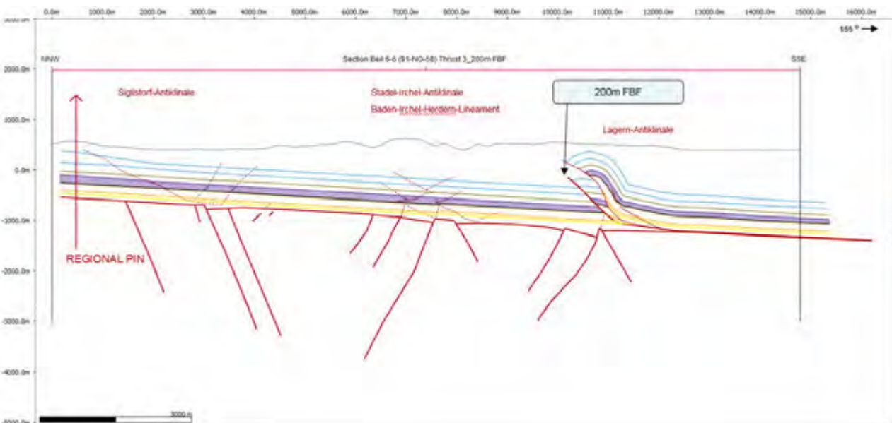
Figure 4—29: The Nördlich Lägern section (based on Section 91-NO-58, Beilage 6-6 in NAB 14-105) with a 200 m displacement along thrust 3 using the Fault-Bend-Folding algorithm. The step causes further steepening in the hanging wall and formation of an additional thrust, but does not cause a fold/drag in the footwall. In detail the fold shape is not as tight as the present-day fold (cf. Figure 4—21). Some pre-thrusting folding is suspected (because of the existing footwall fold, and thickened salt layer).
