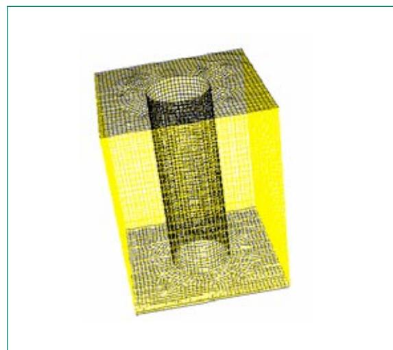
Fig. 1-3: A unit volume in the BWR lower head (312.6 x 312.6 x 400 mm).
