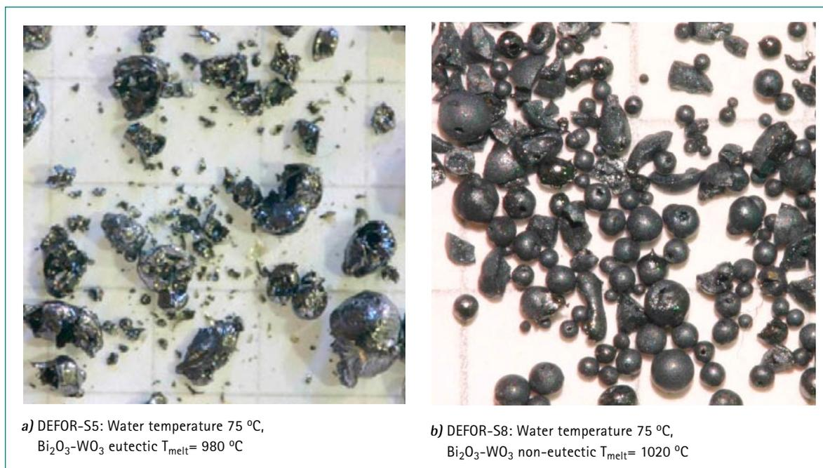
Fig. 2-2: Influence of melt composition on particle morphology (low water subcooling).
